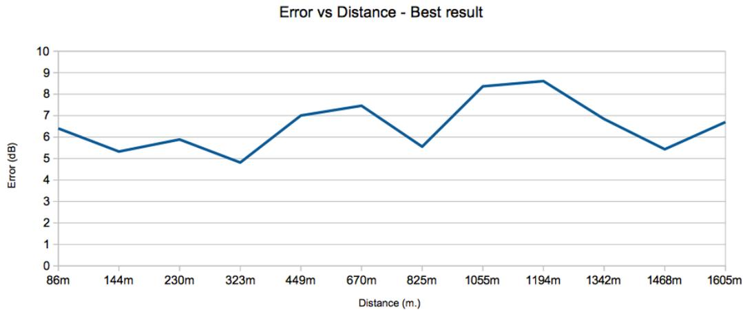
Figure 4 – Error evolution with distance for the best propagation model configuration
